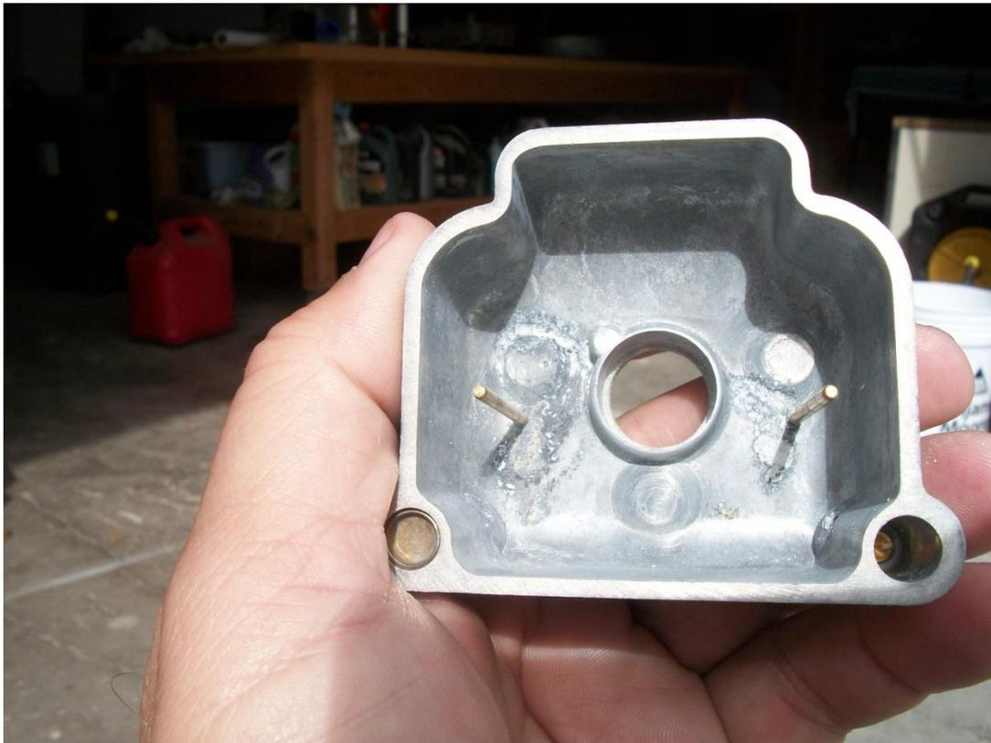
The photo above is out of a 914 powered Europa. Over three years (aircraft flown little in the winter) using mogas high test 92 octane with less than 10% ethanol.
