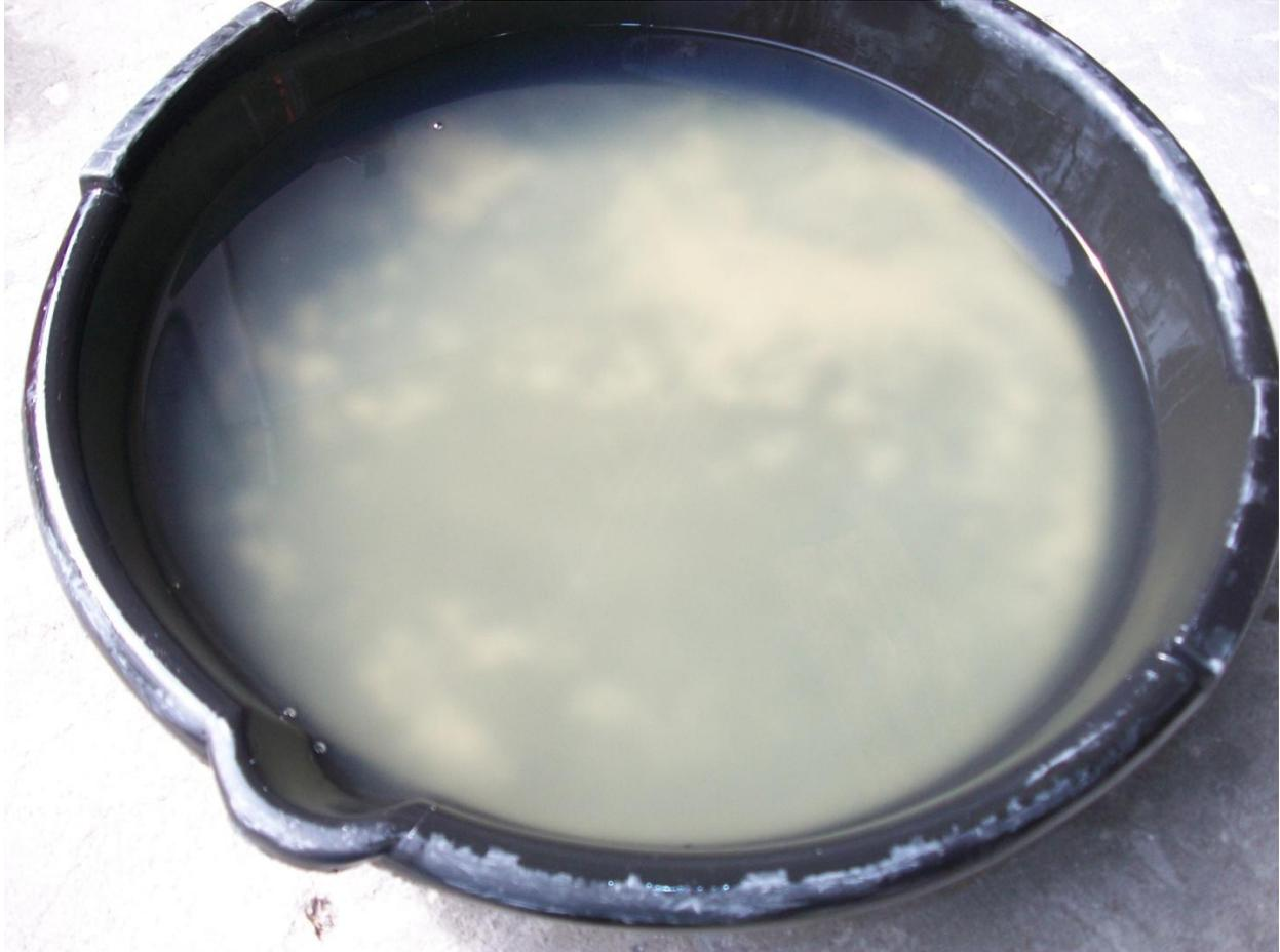
The white clouds are ethanol and water globules in the fuel. Eventually this fuel will clear up and form a water layer on the bottom of the tank. In the water, with ethanol as a food source, a brown fungus has been known to grow on the tank sides and clog filters.
