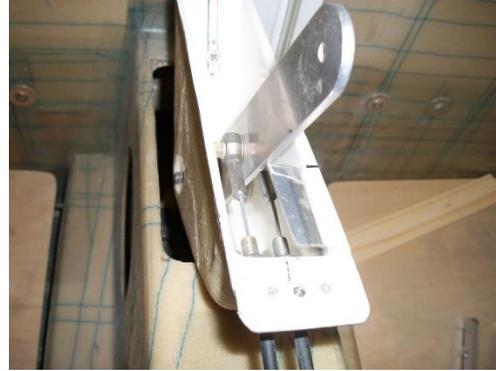
Once installed in the airframe but not hooked to the carb throttle, the cables should move smoothly in and out. With no spring to pull the carbs forward, this will tell if your throttle run is free from binding. If all works well prior to cable to carb connection, you will have trouble free operation.
