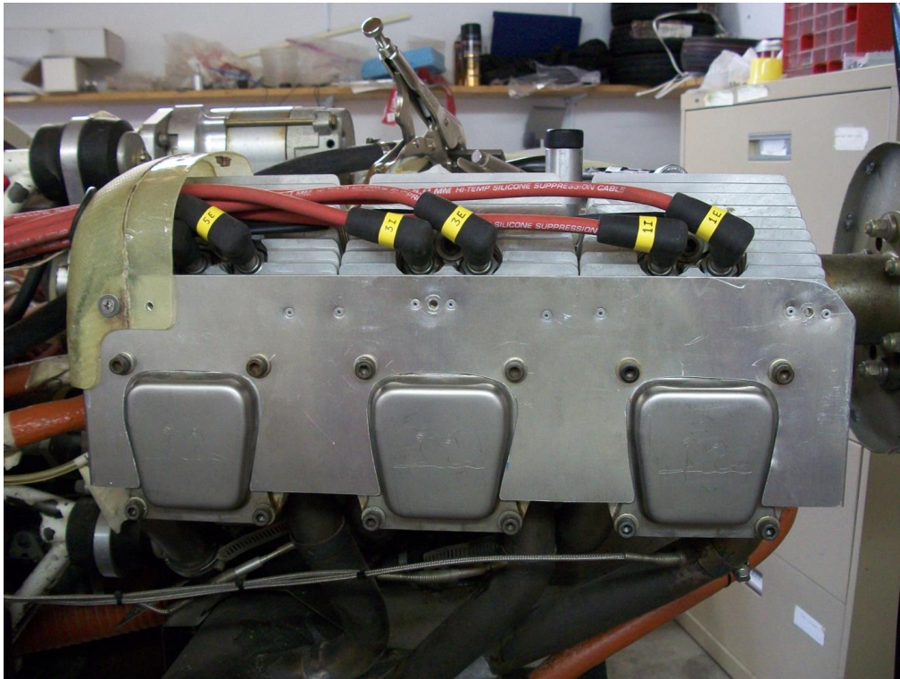
Figure 17. First a metal side skirt was fabricated to attach the lunch boxes to the cylinders. The metal side skirt allowed the attaching screws through metal solidly to the cylinder heads. The sheet metal work is extended a bit lower on the cylinders to deflect more of the air down through the head fins in an attempt to improve flow and dissipate more heat. The fiberglass lunch box plenum is attached to the side skirt via nutplates, screws and sealant. Note no beneath the cylinder ducting is provided.
