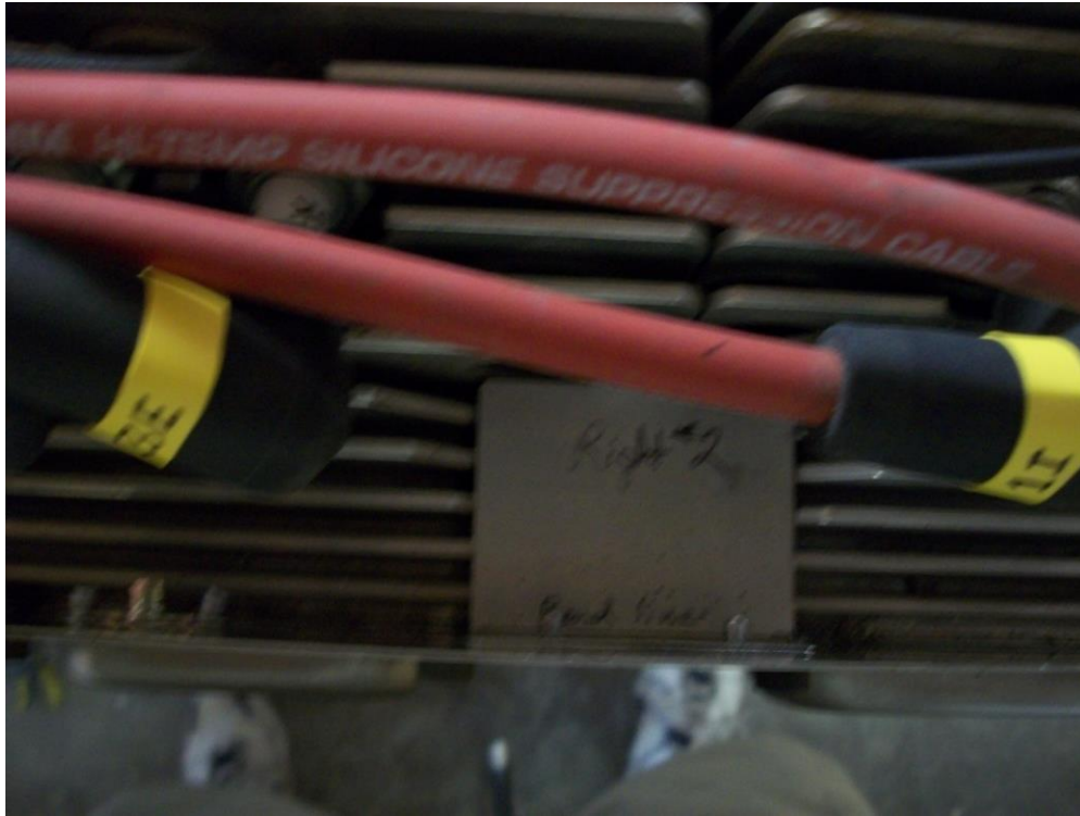
Figure 19. Small air dams were placed between the cylinder heads where the oil galley connects to the heads so as to block any air exit about these 1 inch sized holes. All air goes through the cylinder fins. The metal sheet makes it very easy to attach and adjust these vanes and gap seals.
