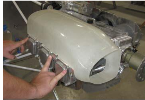
Figure 6. New Factory Plenum
