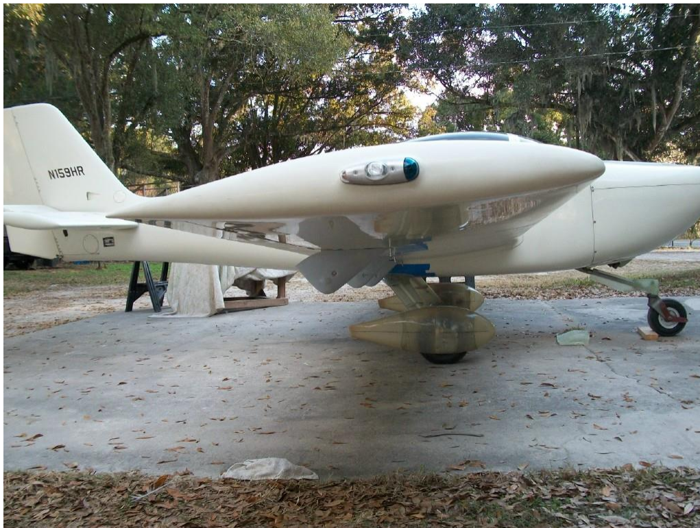
Figure 23. Note that the first attempt at a cowl exit ends about the same point as the exhaust stacks.
