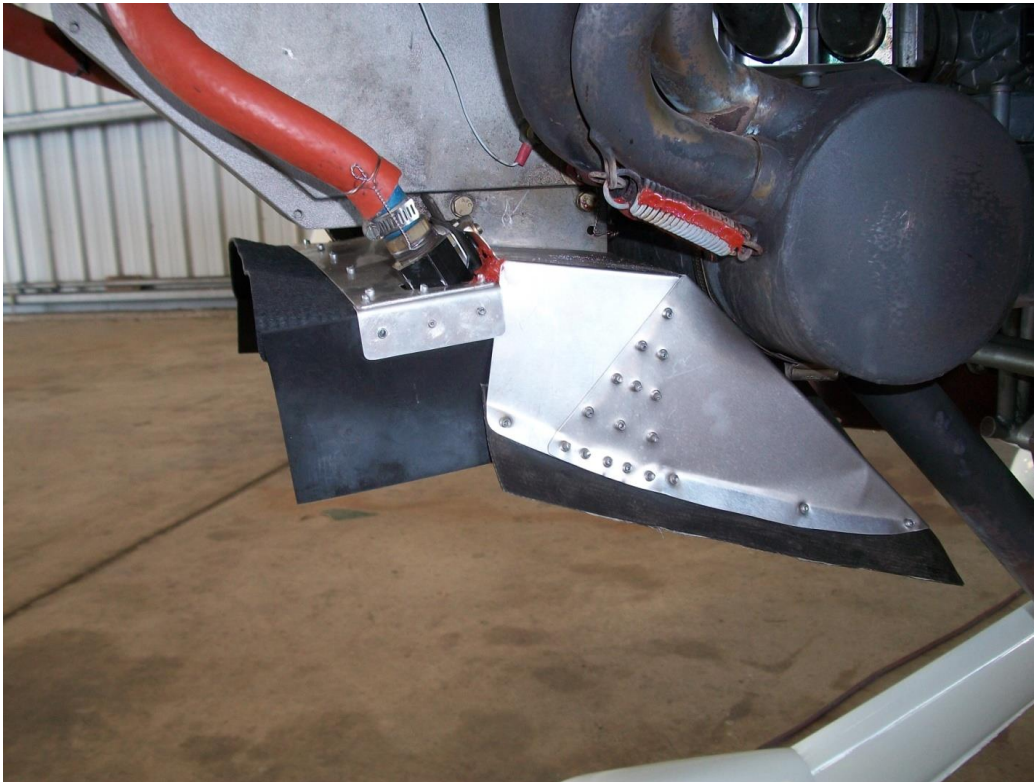
Figure 22. Oil cooler ducting was angled down and aft slightly and sealed completely with metal and cowl seal and sealant to the duct and cowl floor.
