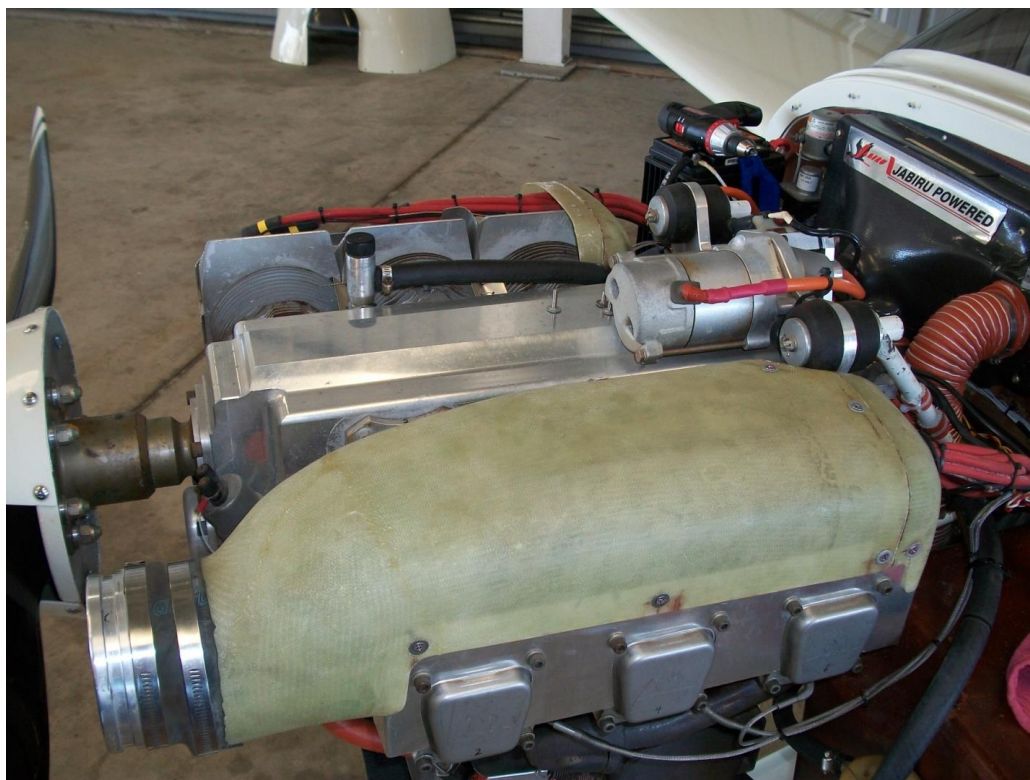
Figure 18. The new fiberglass plenum is installed using 5 screws and one spring on the inboard side. The aft section is held on with one screw. This makes for very easy access and a good foundation for cooling deflectors and seals.
