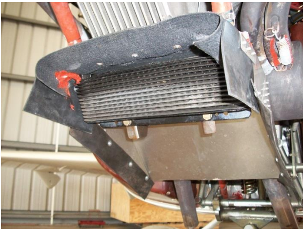
Figure 14 and 15. As can be seen in the above photos, the metal duct is sealed tightly, and the photo on the left shows how the lip of the oil inlet and the cowl exit ramp were included in the cowl to still leave the cowl pleasing in shape. However, all was not well initially.
