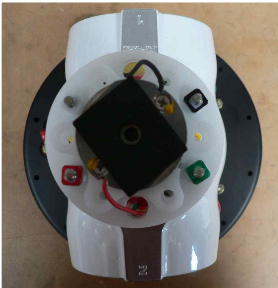
Figure 19. Location of Adjustable Pitch Stops on 2-bladed Propeller Hub Assembly (AP420 shown)
