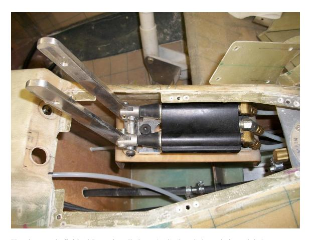
Here is a nearly finished Jamar installation. Again the whole cockpit module is reinforced and a flange made to install the top cover. The Jamar brake cylinder is secured with Allen head tapered bolts for a nice fit and finish. Use a magnetized Allen wrench and you don't drop the crews into the dark hole underneath.
