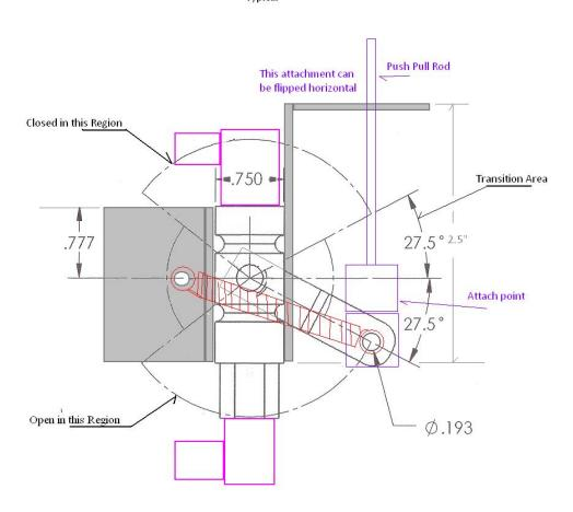
Shown below is a mockup of a Matco set of cylinders with the park brake sticking up from underneath with a push pull positive release and spring loaded up and down position park brake.
