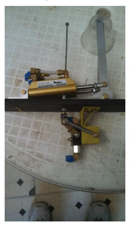
Below is the Matco installation using a detachable panel in the top of the cockpit module showing the C panel glassed to the module side.
