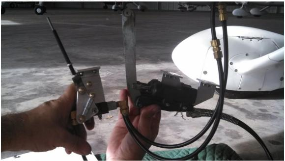
These brakes are easy to make but must be leveled and filled when the pads wear, or you have spongy brakes as there is no reservoir to compensate for pad wear. No reservoir also means a small leak leaves no brakes at all. The manufacture is cheap and normally a 9-10 inch handle from lower pivot to top knob gives good pressure and are easy to pull for normal operations.
