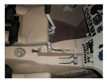
The Kart brake handles are 1.5 inches apart so space is limited and putting knobs on must be planned. The small tab at bottom aft and below the brake slot is the access for fluid servicing. However, I have found that getting the bubble out of the master still requires loosening the brakes master and rotating it forward to level to get the master topped off absolutely full to the top. It is messy also, as Mil 5606 or the Dot fluids stain the interior.
