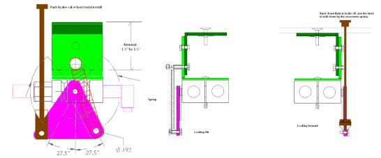
To install brake valve in horizontal position it is recommended a triangular shaped part be attached to the provided arm and attach the vertical pull rod to the third leg as shown to allow a spring and the rod to work with the proper valve angles.
