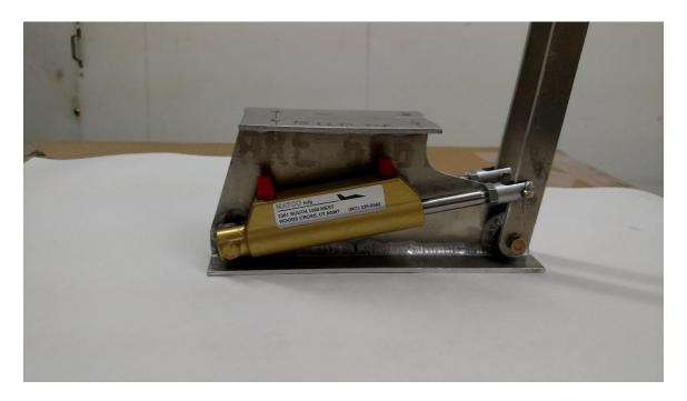
This is a design that does not include an integral park brake to fit between the handles or near them. I like a separate location for the parking brake valve, but we have fabricated an all in one holder out of sheet metal, angles etc. for those who must have the brakes as a unit. A bit of a Rube Goldberg project: "Never make anything simple if it can be made complex and wonderful".
