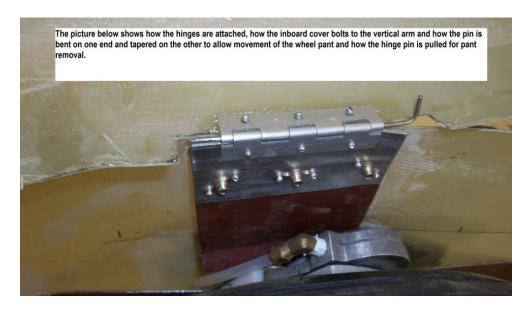
On some installations, the hinge is not riveted to the bracket but is secured using the riveted nutplates. This is a slick install also but more eyeball work is needed. See photo above.
