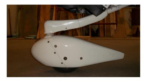
On the left side one can see the nose cone cut is quite raked aft. It is raked to allow the nose cone to open via three screws and pivot to allow access to the valve stem. Be sure to install the tire with the valve stem on the left.
