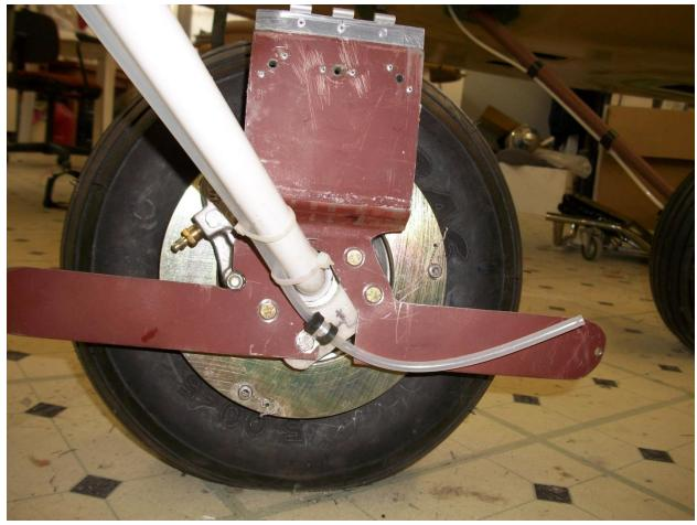
Once the bracket is bent to allow clearance, it is time to attach it.
