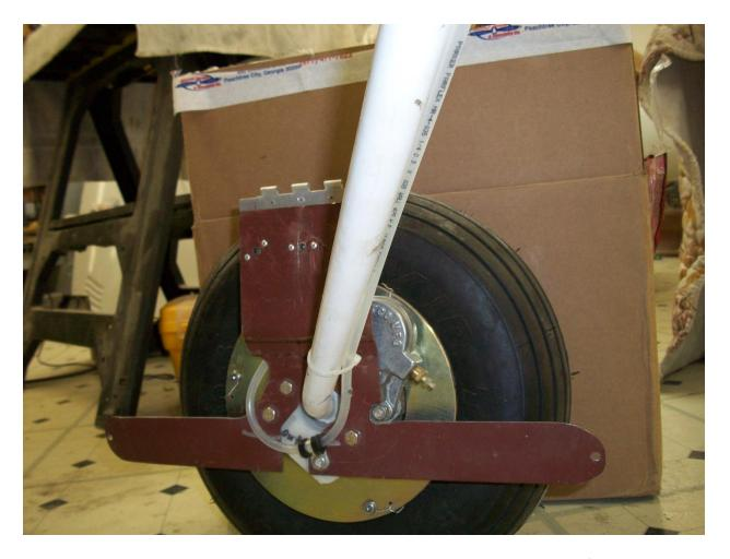
More than one Adel cushion clamp may be necessary to provide adequate clearance. If the brakes are worn, it is necessary to manually move the brake caliper out to its full compression to assure the metal bracket does not push against the caliper.
