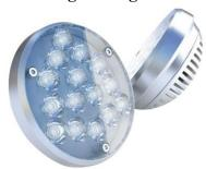
Aveo Engineering has a landing/taxi (bright/dim) option and are of excellent quality. At \$755 they are very expensive, but the pattern and low amperage are acceptable. Taxi, Landing and both beams draw only 15/46/61 watts or at 12 volts 1.3/4/5 amps. It has a hot center beam and a dim for taxi. It is very large for a Par 36 but very good.
