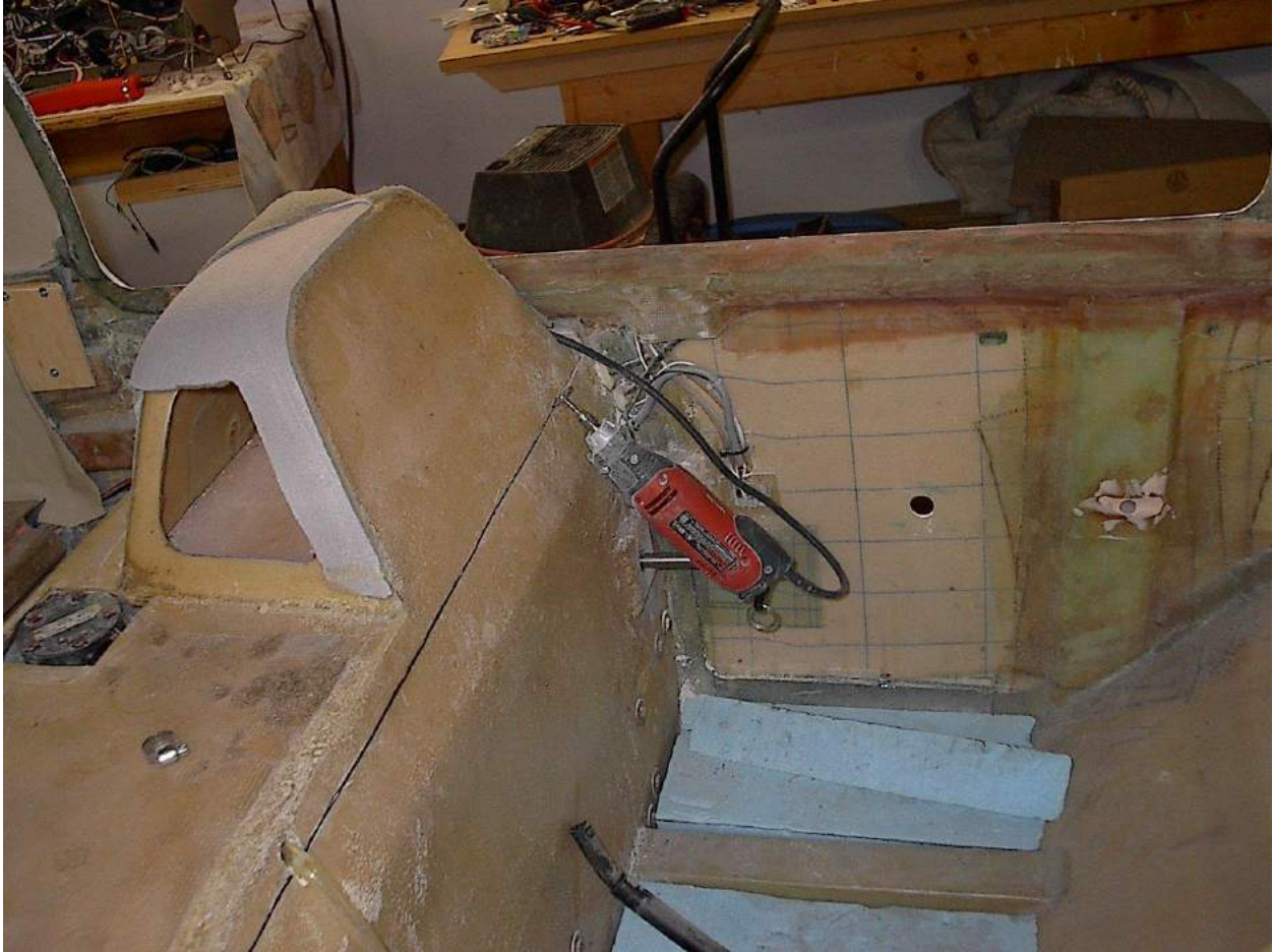
Figure 2 Initial cut along front of the cockpit just above the break in the cockpit. I could have gone lower in the front to within 1/2 inch of the break and still had ample room for the flange later to be added during the top reinstallation.
