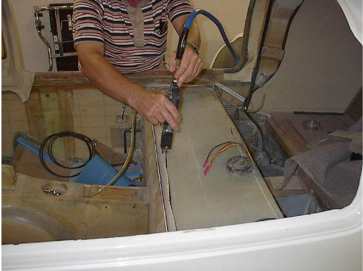
Figure 5 Cutting the top out of the tank.
