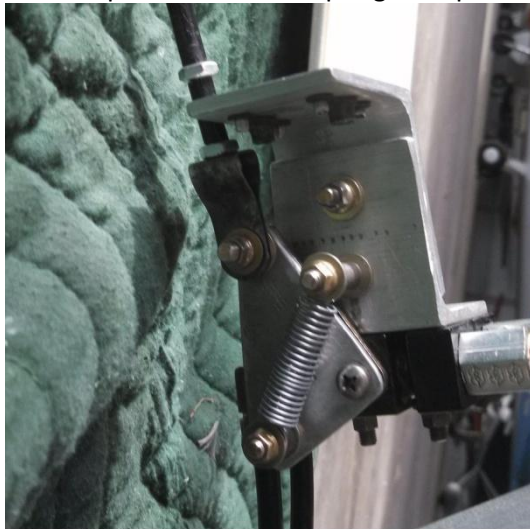
To install brake valve in horizontal position it is recommended a triangular shaped part be attached to the provided arm and attach the vertical pull rod to the third leg as shown to allow a spring and the rod to work with the proper valve angles.
