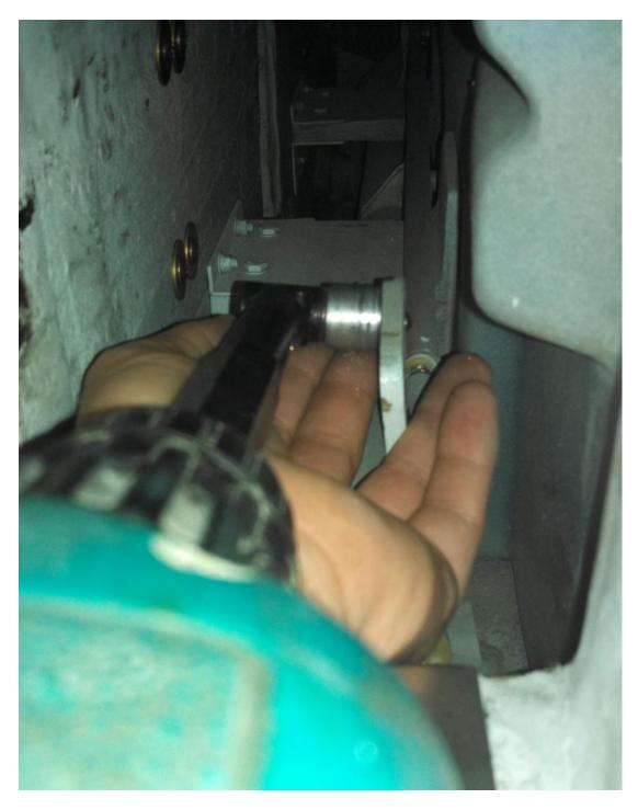
As can be seen in the photo above, clearance is tight but the spacer keeps the head flat against the aluminum and the pilot of the bit does the rest of the work.
