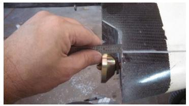
If you find yourself with the problem above and are concerned with clearance, remember that the additional root glass layups will fill this void between the root and pin flange. However, if clearance is still tight between the root and socket, contact tech support and we will supply a non flanged pin.
