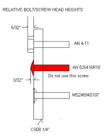
In the event there is a clearance problems using the AN4-11 bolts remove the CS08 and countersink the CS08 for the MS24694S107 countersunk screws. Removal of the CS08 would involve the following:
