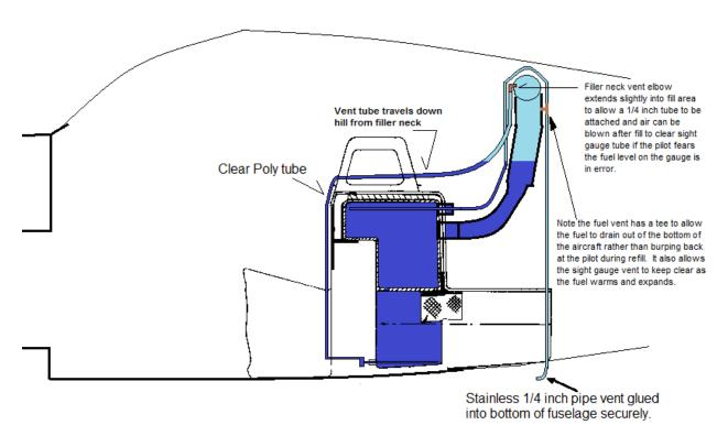
Second, the supply or bottom side of the sight gauge must not be located in a feed or return line or fitting. Any flow through the fitting will pull or push the level of the gauge up or down as fuel flows through the line or fitting. An excellent place is to hook the sight gauge lower line to the fuel tank drain fitting. Either hook it into a street Tee or brass tee and nipple screwed into the FS09 tank boss at the bottom front of the tank, or into the drain line.
