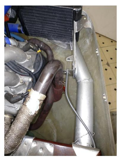
Fabrication for this heater was done by welding an aluminum tube, but the forward end of the tube could be glassed to the cowl and SCEET tube used to enter the cockpit with a stock two inch flanged fitting. In practice, the owner added a top and bottom lip to assure all the heat entered the tube.
