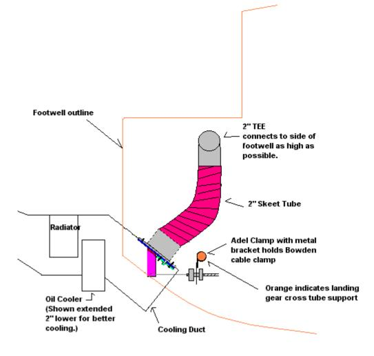
I prefer to make my flapper door as far forward as possible to clear mono firewalls and get the flap/door lip as close to the oil cooler as possible. I also prefer to put a couple of side curtains of sheet metal to direct as much heated air as possible into the 2 inch duct.
