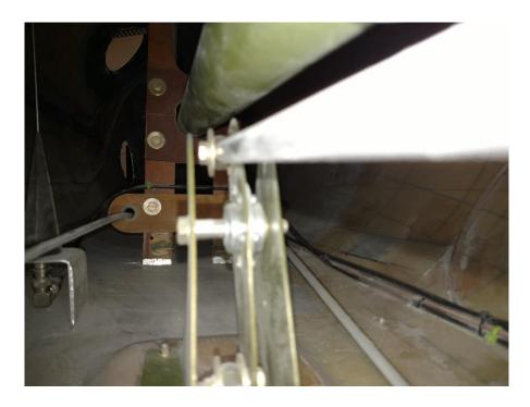
No installation is without effort and to many, not worth the time. The mono makes installation to the pitch tube very difficult, and rear access panel size are the factors which affect the installation type. For most mono owners putting the pitch servo just behind the baggage bay bulkhead on the floor is required.
