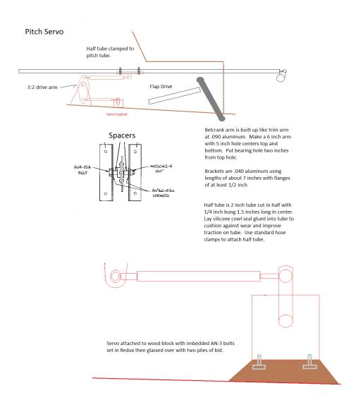
The second method of pitch servo installation is dependent on the access the owner/builder has to the stab pitch tube and tower area. Should the installer have adequate access to the actual pitch tube, I prefer to extend the pitch tube attachment via two pieces of steel sheet to allow a rear mounted direct servo to pitch tube attachment.
