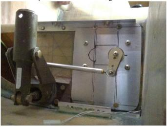
The roll autopilot installation requires an open area normally used under the pilot or passenger seat. Today's smaller servos fit quite nicely into these holes and installation only requires the fabrication of a plate, a cover to prevent control interference, and a bracket installed on the stick. Note in the photo
