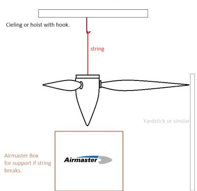
Static Balance Setup Used by CFC, Inc.
