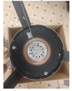
Recheck the propeller static balance after all balancing bolts are installed.
