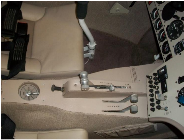
Normal choke with throttle friction shown at left. Modified choke T handle was added for easier choke operations shown on the right.
