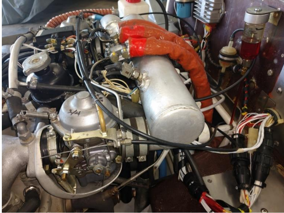
Photo of 12AY showing choke cable runs.
