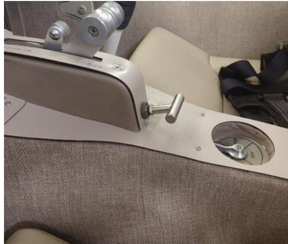
Normal choke with throttle friction shown at left. Modified choke T handle was added for easier choke operations shown on the right.
