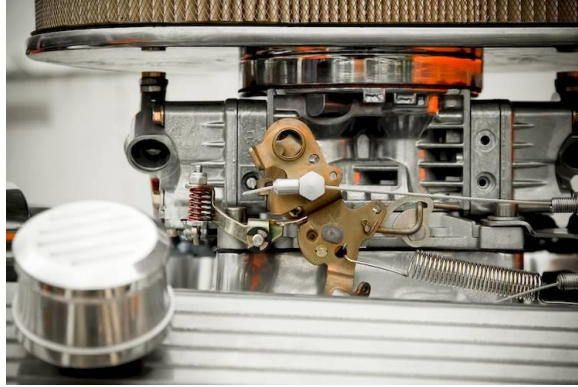
Typical Holley Carburetor throttle cable that traverses 90 degrees of rotation in a hotrod.
