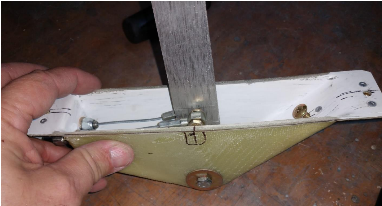
Photo of Bench cables at mid throttle. Note in the photo above the box is marked for cutting to get access to the bolt heads and nuts rather than pulling the handle out to repair.
