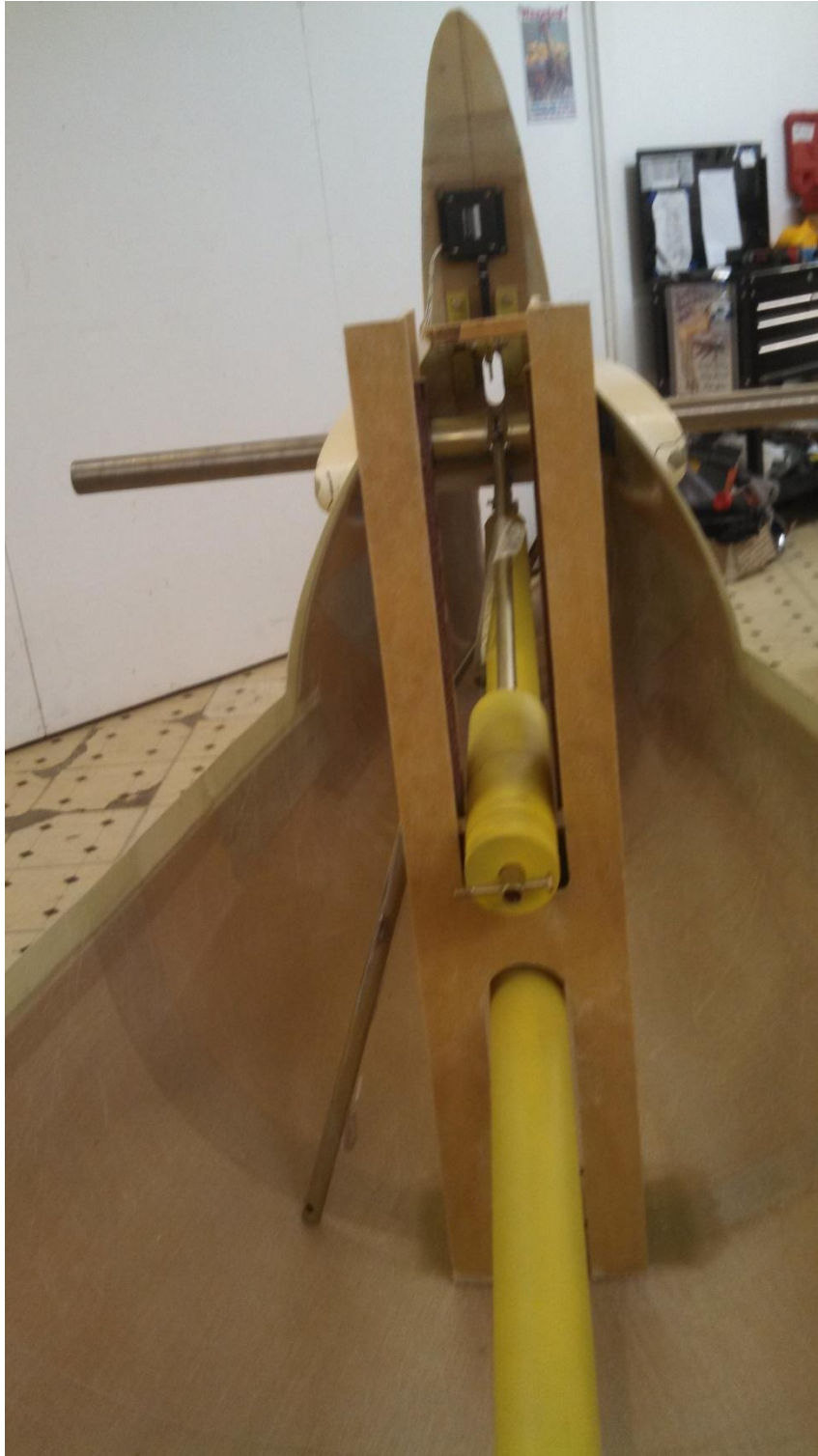
Front view of the trim system and counter weights and the tower installation.
